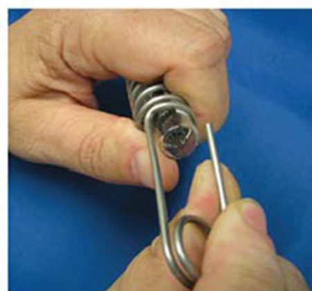
Bending wire to insert WMST™ sampler
