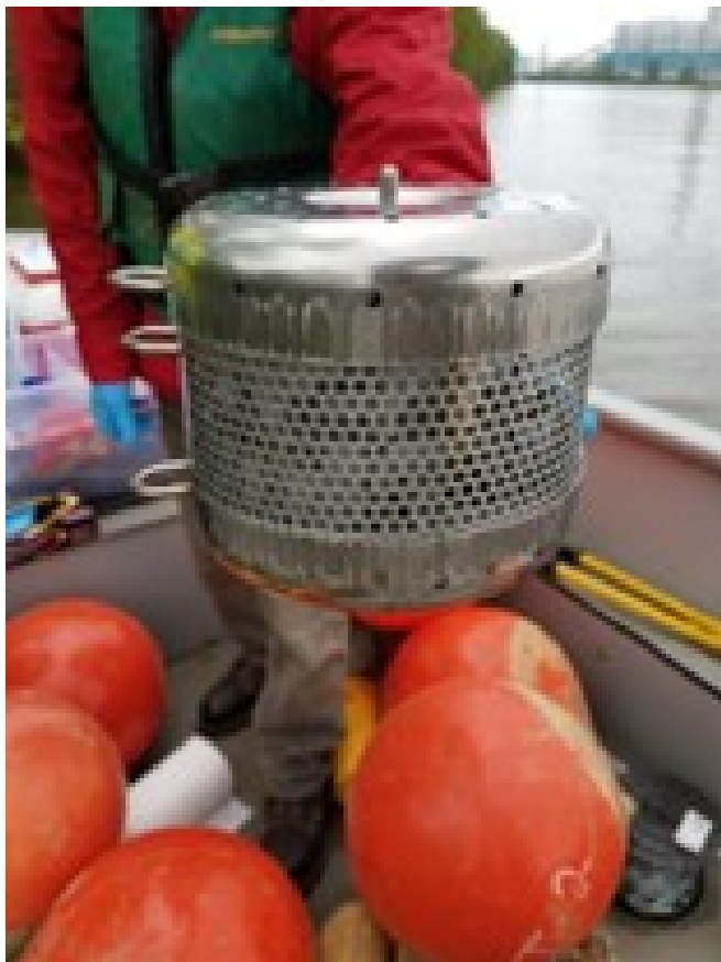
Figure 5-37. A semipermeable membrane device assembled prior to deployment. Source: Anchor QEA, used with permission.
