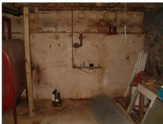
Commercial building basement, two AGI Universal Samplers Suspended, Summa can on floor; heating oil tank and workbench
