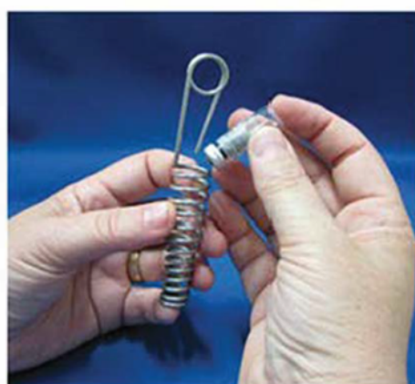
Aligning WMST™ sampler in wire hanger
