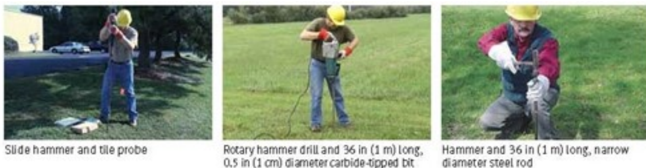
Figure 5-29. AGI sampler installation. Source: AGI, used with permission.
