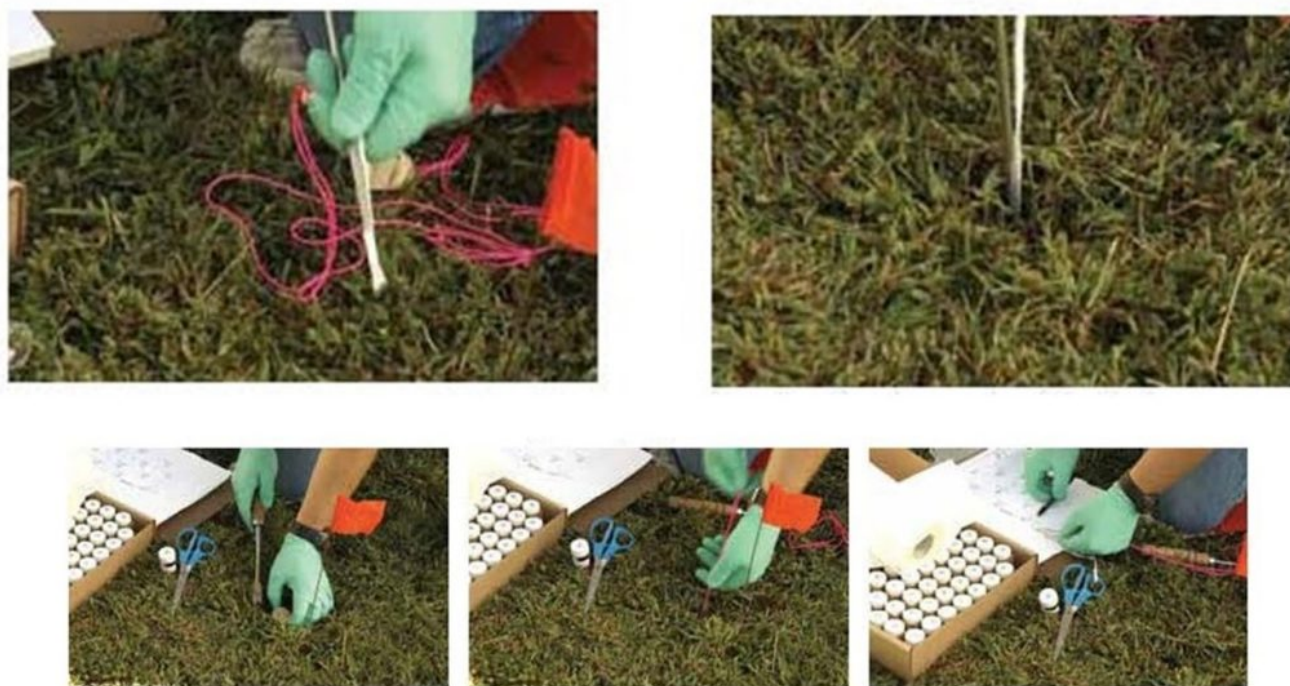
Figure 5-30. AGI sampler deployment and retrieval. Source: AGI, used with permission.
